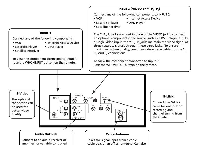
be used for basic component connections.
